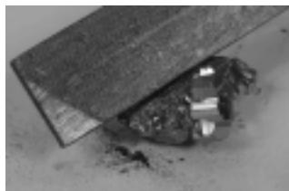
Figure 1: Using a file collect a small amount of fine black pyrite particles. Don't take the particles from the beautiful side of the mineral. There is no need to destroy the nice crystals.
