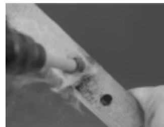
Figure 6: A comfortable possibility to show the principle of a fire drill with a modern drilling machine. With a piece of gun cotton in the hole you will get also a flash.
